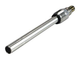
The LDO VISI combine an optical sensor type and electro-optical module in one probe. The sensor has a maximum measurement range of 0 - 100 %  $O_2$ , and a detection limit of 0.03 %  $O_2 / 20$  ppb. It is integrated in a removable sensor cap (OEC), which can easily be exchanged. These exchange caps are available
